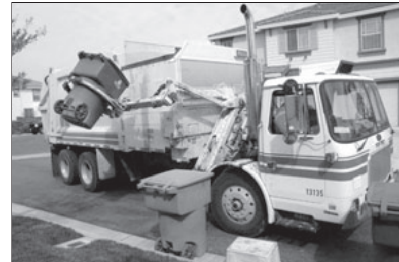
Trucks like the one above use mechanical arms to empty toters. This automated service is used by most of the cities around Vallejo. Vallejo may soon have this service in our neighborhoods.
